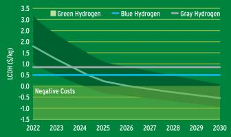
Note: Assuming natural gas price of \$3/MMBtu. Green hydrogen is powered with dedicated solar power. LCOH=levelized cost of hydrogen. Source: Citi GPS, Citi Research Estimates
