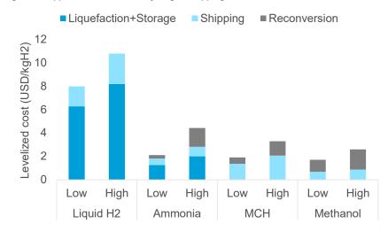
Figure 32. Approximate Levelized Hydrogen Shipping Costs in Different Forms of Carriers
